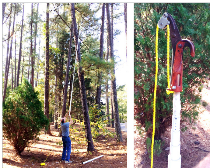
Figure 3—Long-reach pole pruner constructed by attaching a pole pruner cutting head to a ~12-m telescoping tree height pole. (Photo by Tom Christensen)
