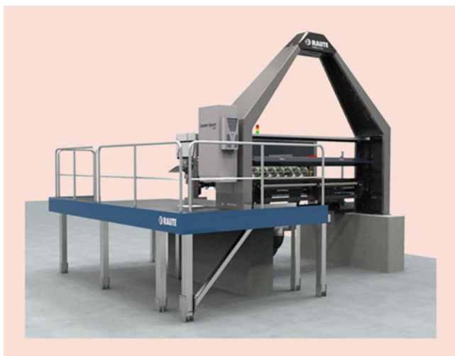
Fig. 20.19 Veneer Visual Analyzer is showing cross grain area or dense knot row for Veneer Strength Analyzer (see chapter veneer grading after drying)
