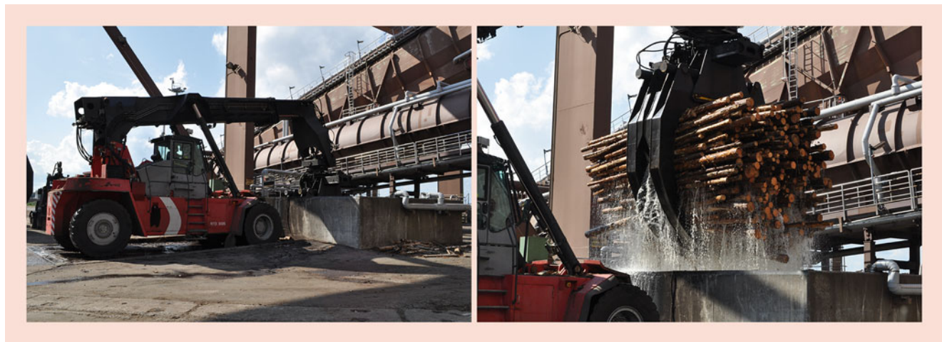
Fig. 20.3 Xylometer measurement of pulpwood in Finland by weighing in the grip above and under the water
