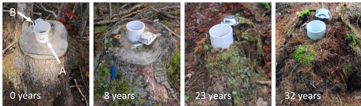
Fig. 1. Examples of Picea rubens stumps used in a chronosequence of CO 2 flux, showing stumps 0, 8, 23, and 32 years since harvest. Images show PVC collars (A, 10 cm diameter) used for CO 2 flux measurements, as well as adjacent reflective solar covers (B) shielding the iButton temperature sensors.
