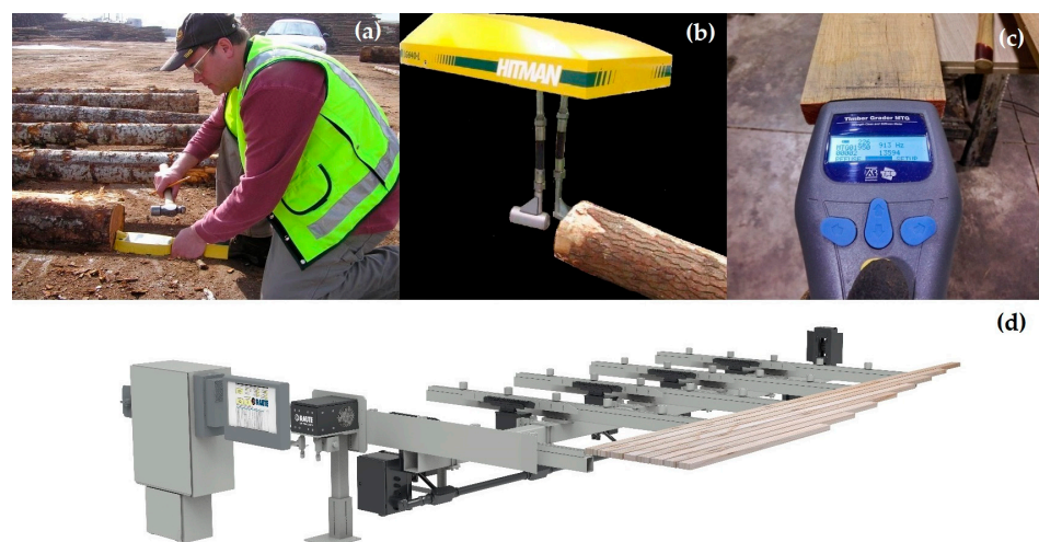
Figure 19. Examples of resonance acoustic-based equipment used in the forest products industry: (a) Portable resonance acoustic tool for log testing (Hitman HM220). (b) In-line automated acoustic log sorting machine (Hitman LG640) (Photo credit: Peter Carter). (c) Portable resonance acoustic tool for sawn timber testing (MTG 960) (Photo credit: GICM-UPM). (d) An in-line acoustic lumber grading system (Lumber Strength Analyzer—Sonic, Photo credit: RAUTE Metriguard Technologies, Inc., Pullman, USA).
