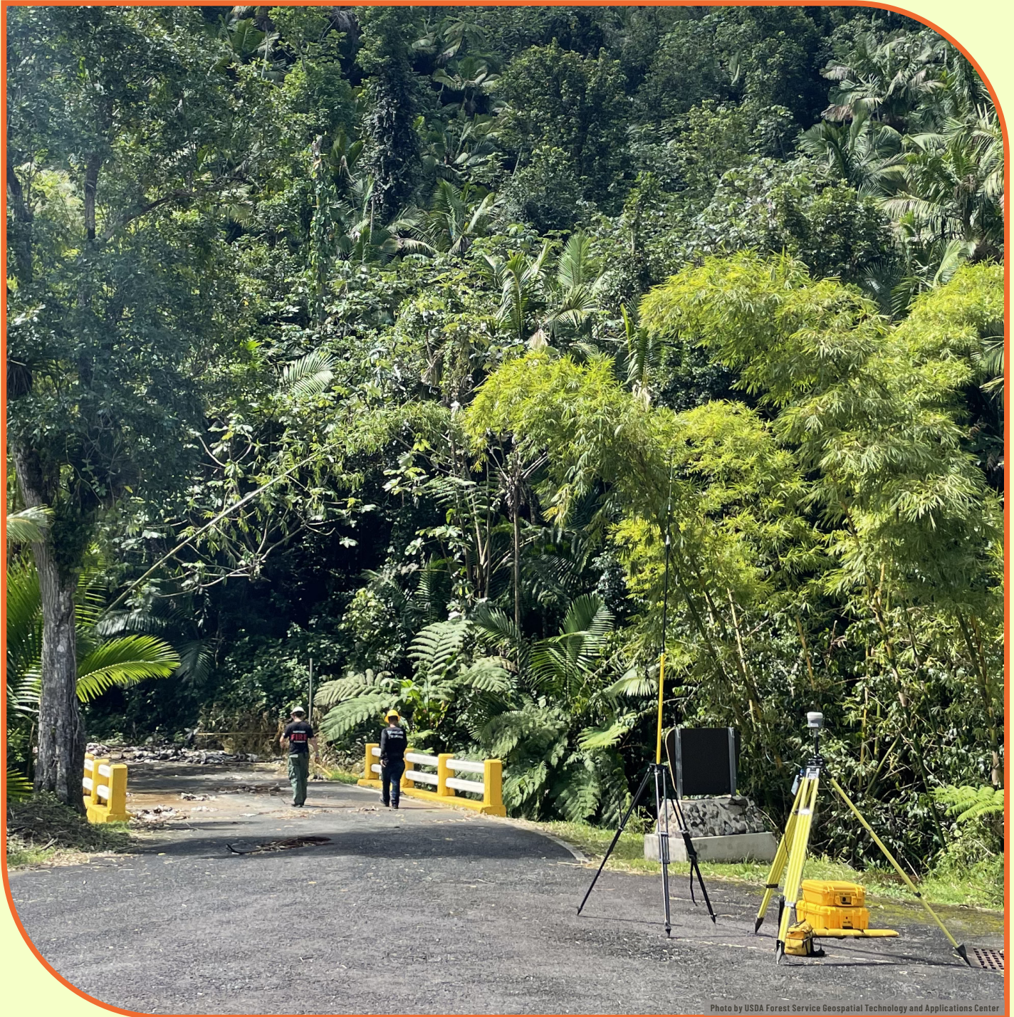
Geospatial Technology and Application Center (GTAC) Set up GPS base stations for surveying a road damaged by landslides to support road repair work.
