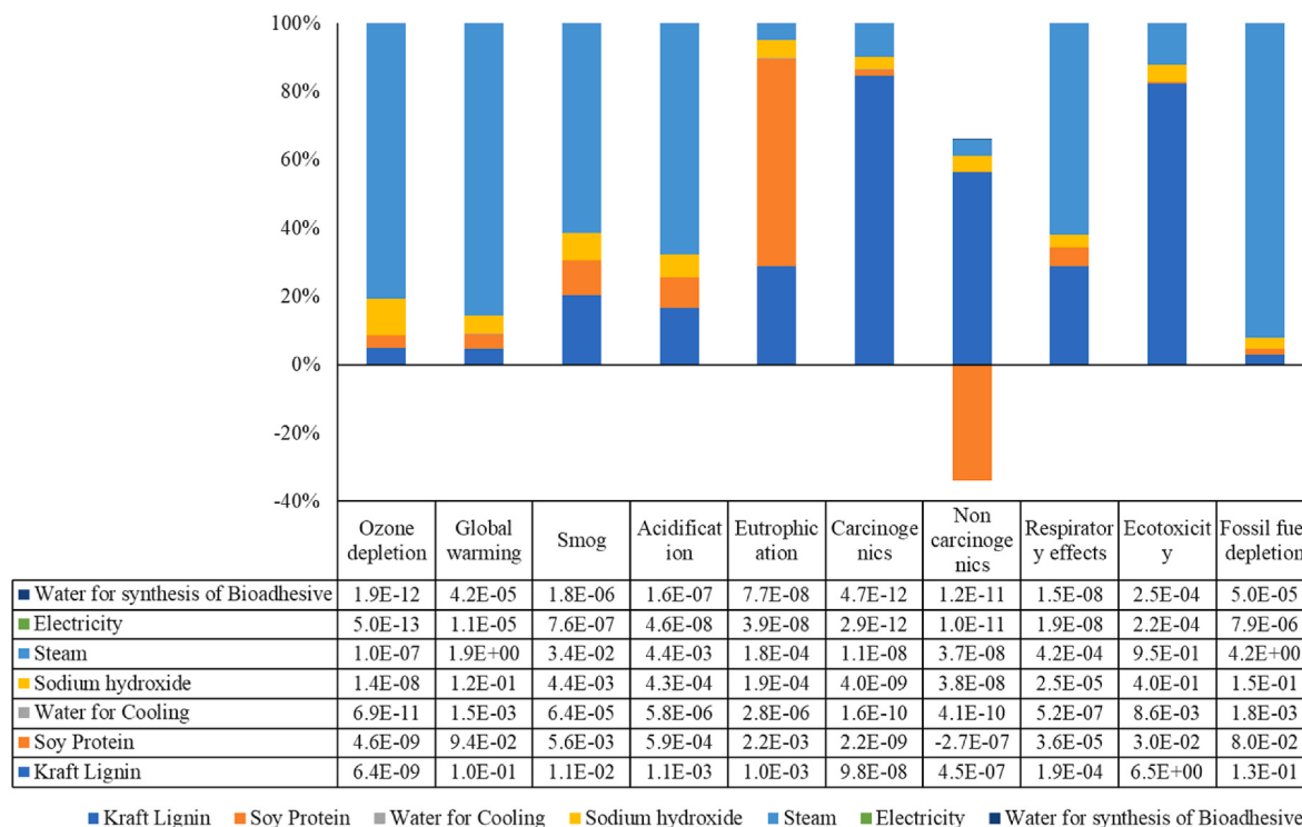
Fig. 6. Life cycle assessment contributions for cradle-to-gate production of 1 kg of lignin-isolate soy protein bioadhesive.
