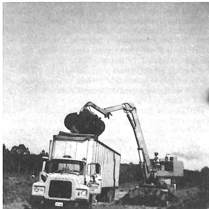
Figure 4.—Chips being loaded into a van; vans require roads that are in relatively good condition.
