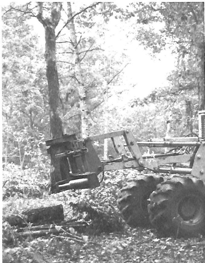
Figure 10.— Hydro-Ax shearing low-quality white oak on Western Highland Rim.
