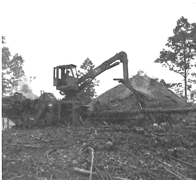
Figure 3.—Tree being fed into chipper; chips are being piled before loading.
