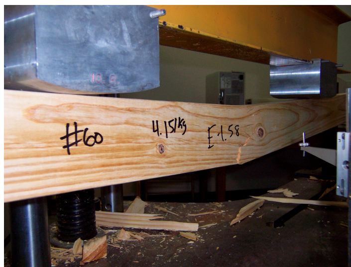
Figure 1. Destructive testing of a 2 \times 4 lumber in edgewise bending as per ASTM standards.
