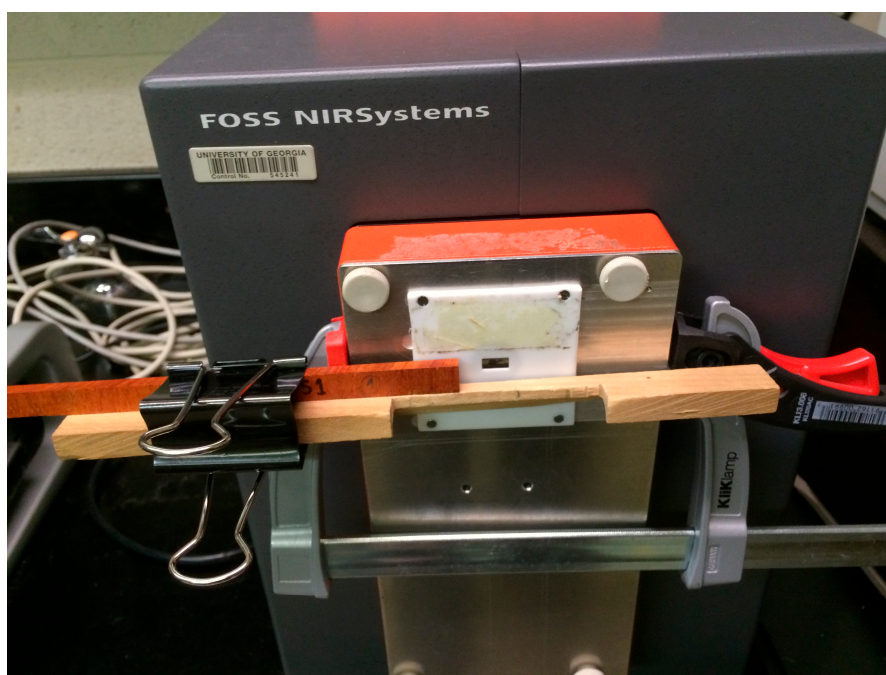
Figure 2. Acquisition of diffuse reflectance near-infrared spectral data from a wood sample on a FOSS NIRSystems Model 5000 scanning spectrophotometer.
