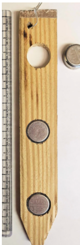
An iButton stake that will measure soil depths 5, 10, and 15 cm when installed with the top of the stake 2 cm below the soil surface. USDA Forest Service photo by Matthew Dickinson
