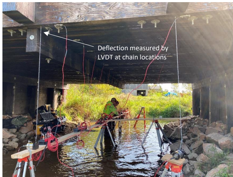
Figure 7-1 Deflection data collected via LVDTs
