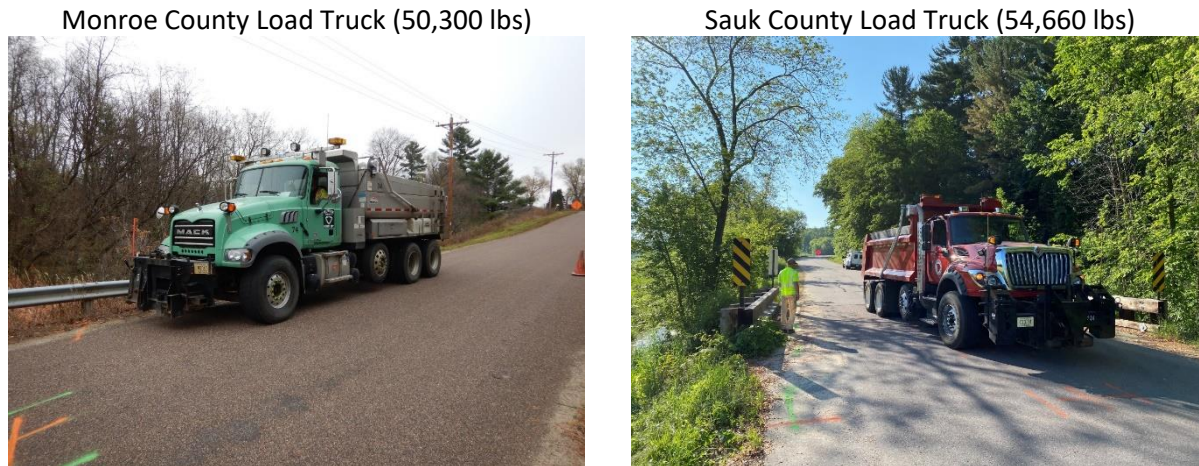
Figure 4-50 LRFD Bridge Load Vehicles
