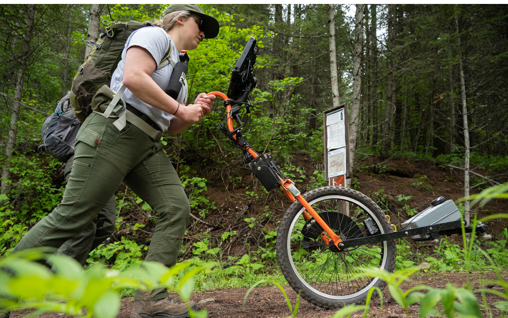
The High-Efficiency Trail Assessment Process (HETAP) machine measures trail attributes that can affect a user's ability to navigate the trail. National Park Service photo.
