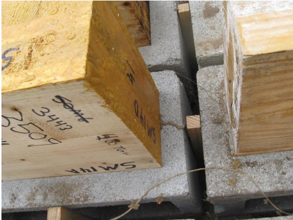
Figure 3: Example of termite activity in test subplot. Mud tube observed from feeder stake to test sample
