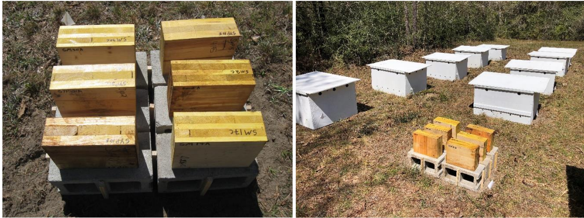
Figure 1: Placement of CLT test samples on cinder blocks and position of some of the feeder stakes (left). Test plot showing subplot before covering and other test plots with ventilated covers
