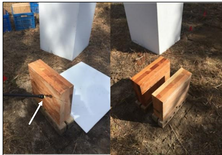
Figure 3: Photographs showing the arrangement of ground bricks and mass timber samples in subplots. Treatment with spray-on borate (23% DOT; arrow shows tip of spray nozzle) in the preventative and remedial treatments.
