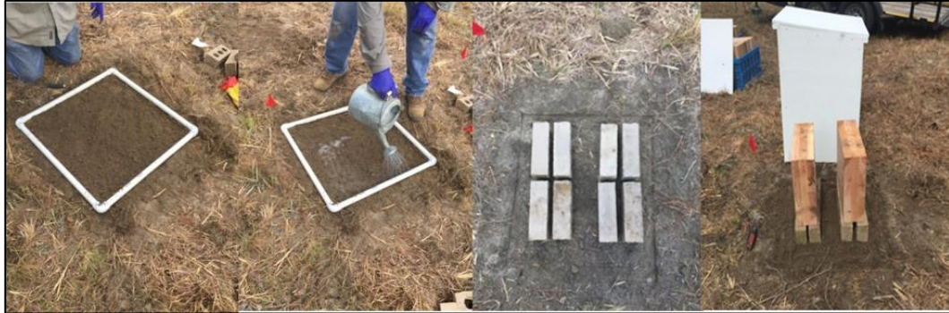
Figure 2: Treatment with fipronil soil termiticide showing arrangement of ground bricks or cinder blocks and CLT in soil termiticide subplots.
