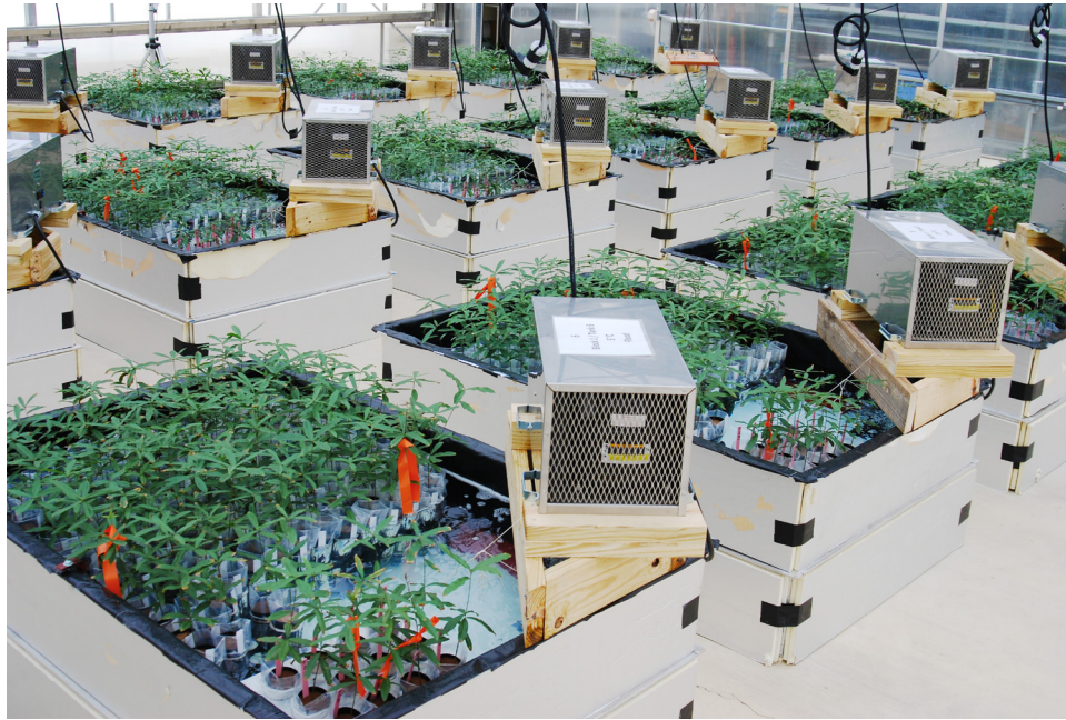
Figure 1—Willow oak seedlings in soil temperature control tanks. Pots in leak-proof plastic bags were placed in tanks to maintain soil temperature within \pm 0.5 °C. (Photo courtesy of Benjamin A. Babst)
