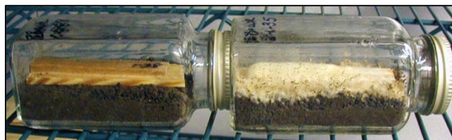
Figure 1—Modified soil bottles after a 12-week test: uninoculated (left) and inoculated (right).
