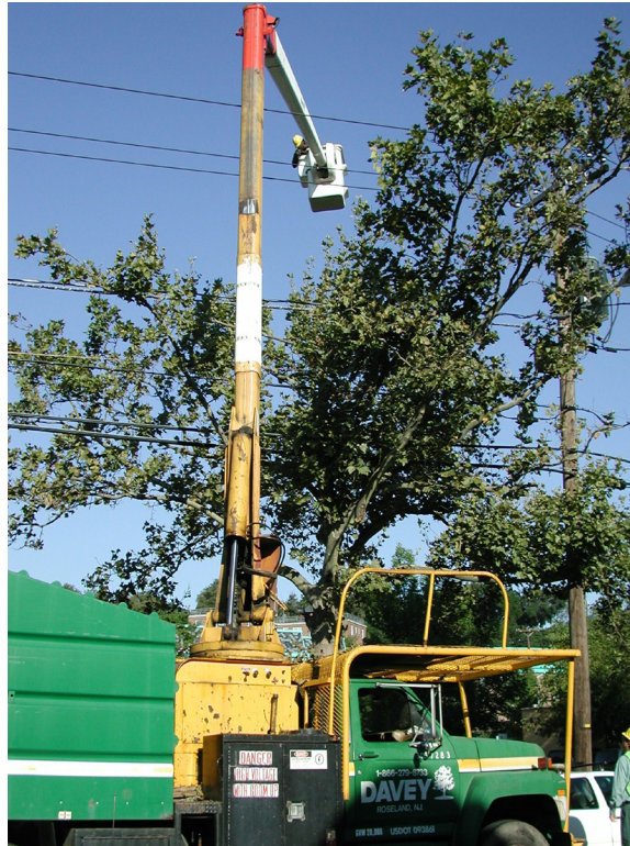
Figure 11. —Lifting equipment such as bucket trucks facilitate canopy inspection surveys. Licensed photo by Thomas B. Denholm, New Jersey Department of Agriculture/Bugwood.org.
