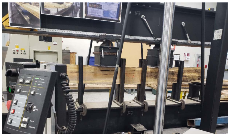
Figure 1.—Bending machine set up with the extensometer attached to the sample.
