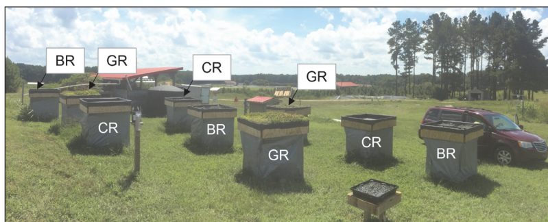
Figure 1. Control roof (CR), blue roof (BR), and green roof (GR) plots at NCSU SECREF, Raleigh, NC.
