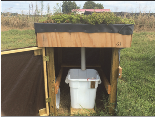
Figure 3. Constructed green roof plot with central drain emptying into runoff storage bin.
