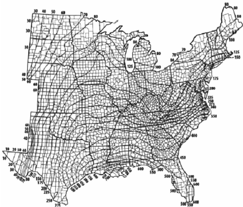
Figure 8 Current isoerodent map of eastern USA (EPA, 2001).
