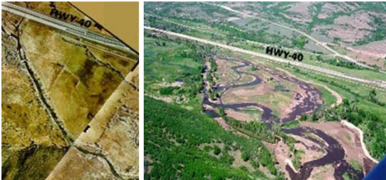
Figure 4.23a-b —Provo River in Utah before (a) and after (b) restoration, which included physical channel restructuring to increase sinuosity. Image from URMCC 2009; used with permission.
