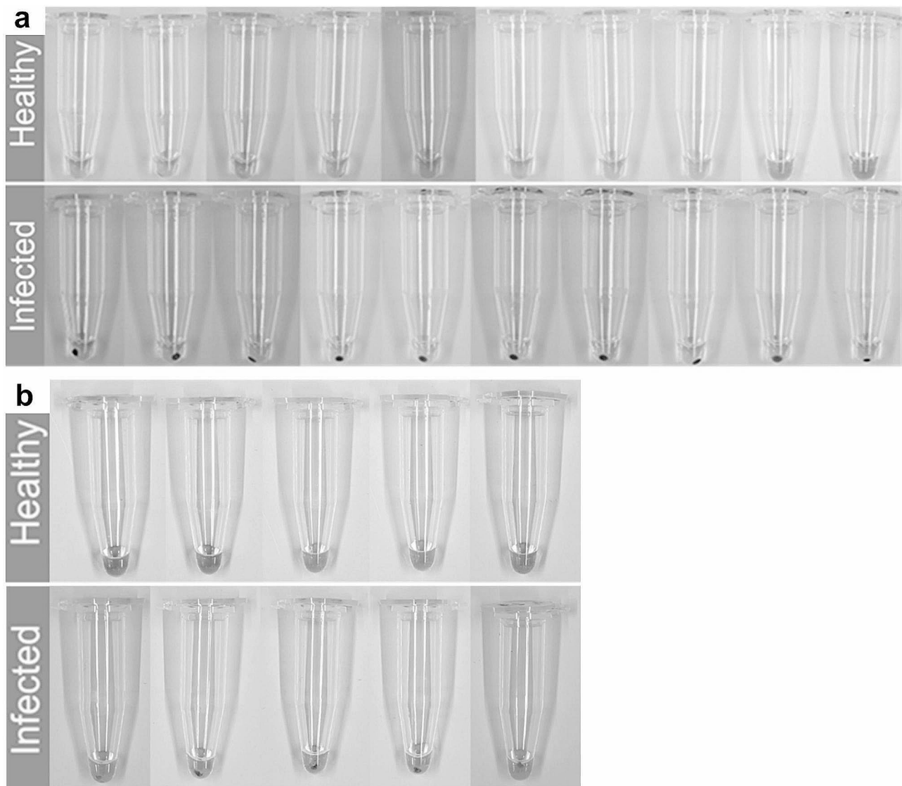
Fig. 7 Detection of the fungus Bretziella fagacearum in wood chip samples from healthy and infected oak trees. After DNA extraction and amplification using LAMP, visualization of the amplicon is performed using oligos-conjugated gold nanoparticles. In the presence of the target DNA, the nanoparticles bind to the DNA amplicons, and assemble into globular nanostructures that can be easily precipitated to form a visible red pellet at the bottom of the microtube. (a) Results from LAMP assay conducted using a real-time PCR instrument, (b) Results from LAMP assay conducted using a portable dry heat block
