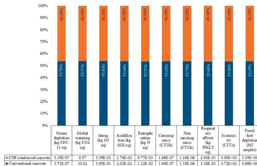
Fig. 7. Environmental impacts of CNF-reinforced and conventional concrete mixtures (functional unit: 1 m 3 /MPa), cradle-to-gate.
