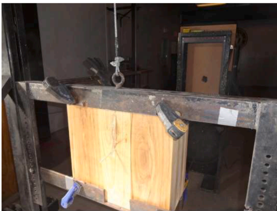
Fig. 4. Test Specimen Mounting for Ballistic Testing [1].
