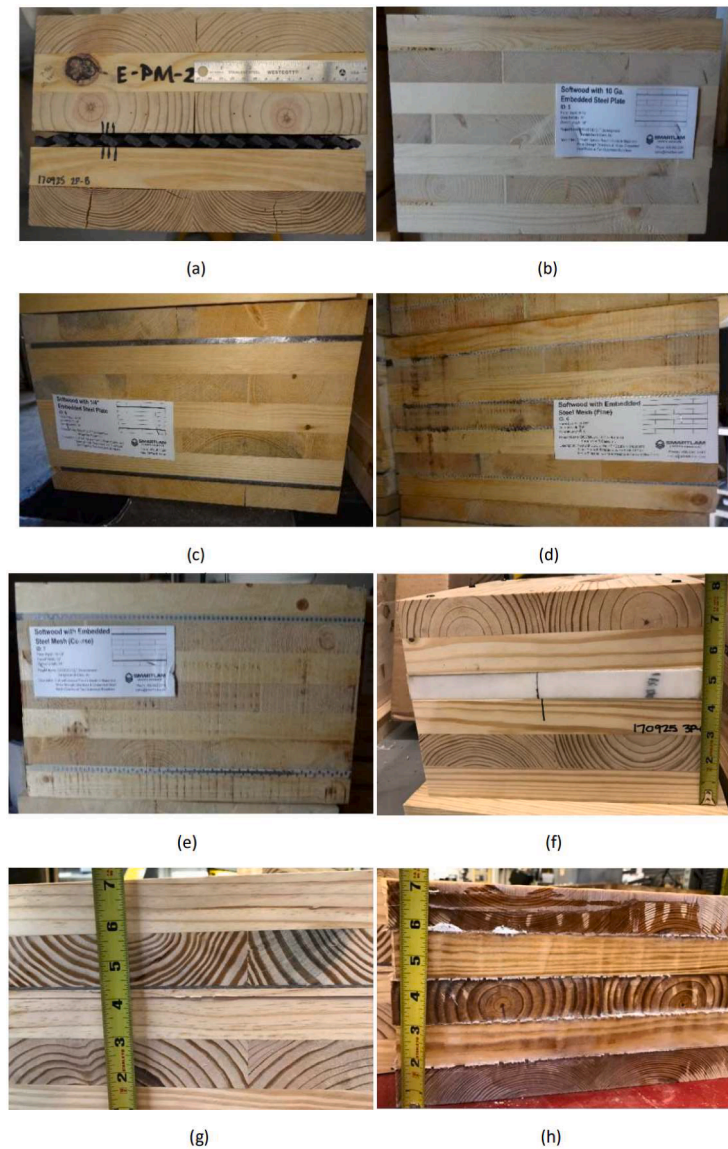
Fig. 2. Example panel configurations. (a) Type 2: Expanded Metal Plate (b) Type 5: Mild Steel Plate (Thin, 2 layers) (c) Type 6: Mild Steel Plate (Thick, 2 layers) (d) Type 7: Steel Mesh (Fine, 4 layers) (e) Type 8: Steel Mesh (Coarse, 2 layers) (f) Type 10: UHMWPE (g) Type 11: Fiberglass Fabric (4-ply consolidated) (h) Type 12: Fiberglass Fabric (4-ply separated).
