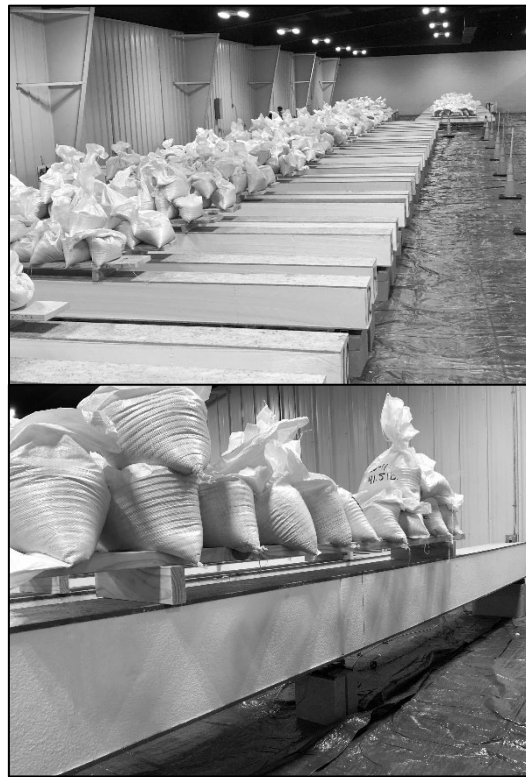
Figure 3—SIPs with loading platforms laden with sandbags for long duration loading (photos property of Mississippi State University).
