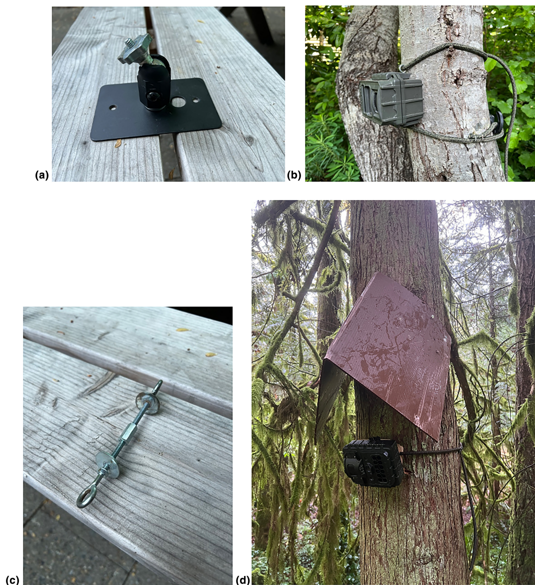
FIGURE 4 Two types of camera-trap mounts that enable a 90^{\circ} rotation of the camera trap: (a) a ball-head, and (b) low-cost eyelet hardware and elastic bands. Also, (c) detail of eyelet hardware, and (d) a camera trap mounted under a corrugated polypropylene roof.
