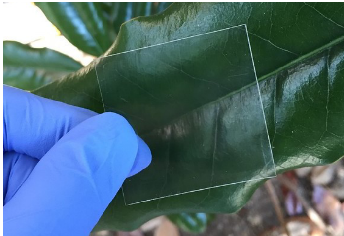
A piece of glass that was made from wood. USDA Forest Service photo.
