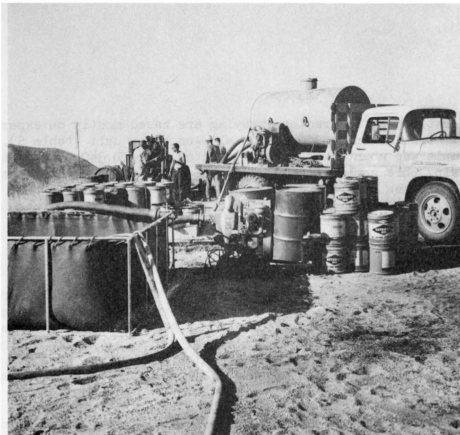
Figure 3.--Costs of a helicopter spray operation include such items as a tanker forhauling water, a canvas water storage tank, portable pump, chemical, and crew.
