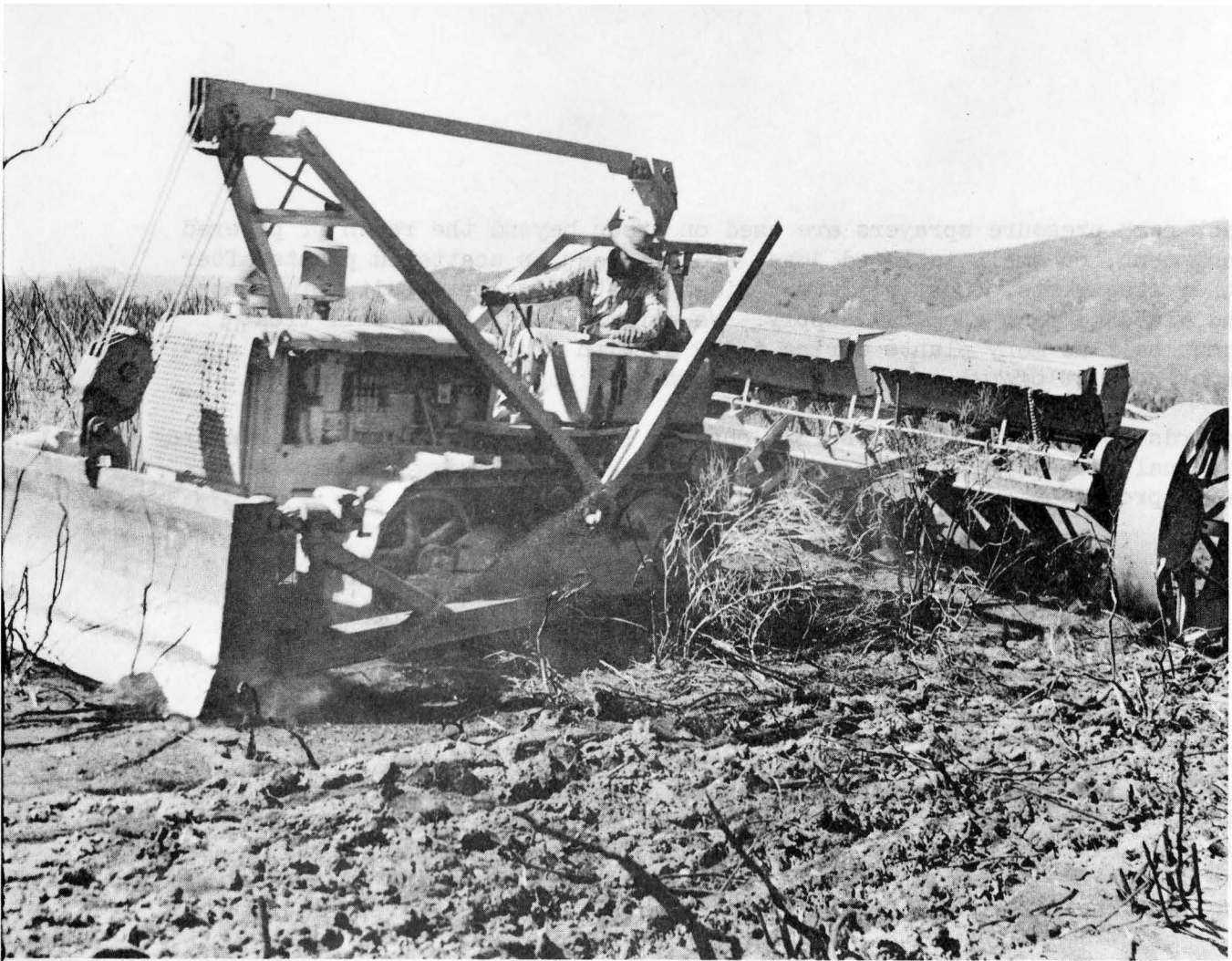
Figure 4.--The rangeland drill is recommended for seeding fuel-break sites.
