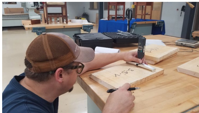
Figure 3—Measuring a sample for flatness. The aluminum brace attached to the indicator allowed the measurements to occur close to the edges of the board.
