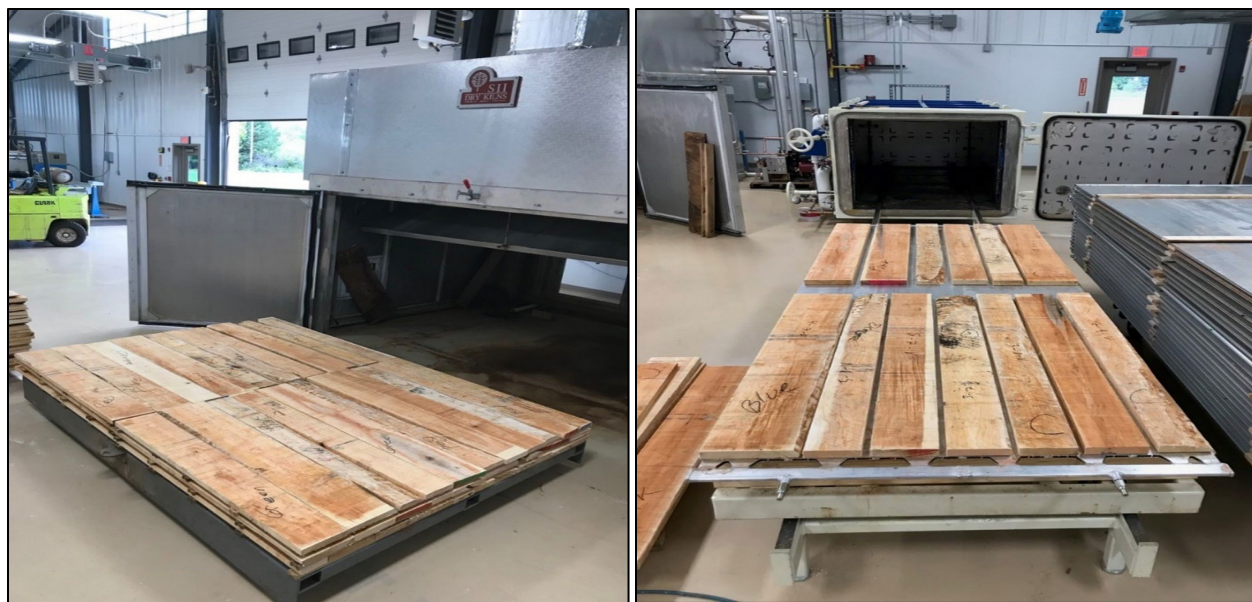
Figure 1—Left: board sample halves stacked on stickers prior to processing in the conventional steam kiln. Right: board sample halves stacked on heating platens prior to processing in the vacuum kiln.
