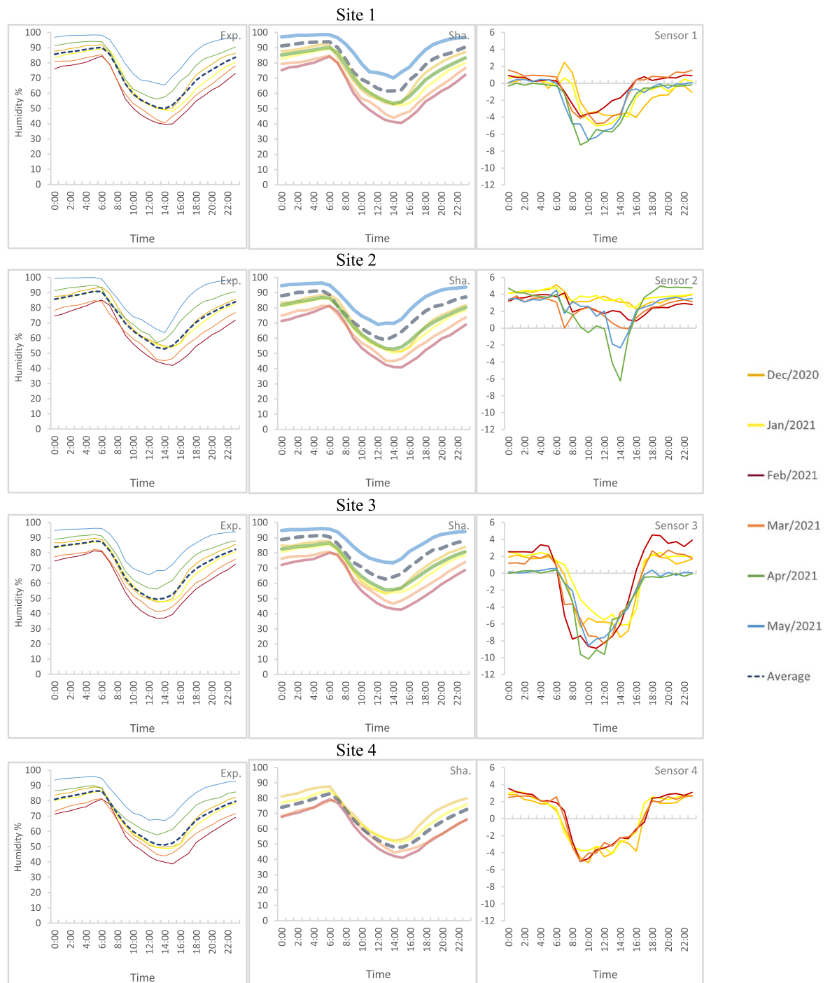
Fig. 4. Hourly humidity cycle for each month (continuous lines, December 2020 to May 2021) by location. Left column: Exposed sensors, middle column: shaded sensors, right column: difference between exposed and shaded sensors. Average values are indicated by dotted lines.
