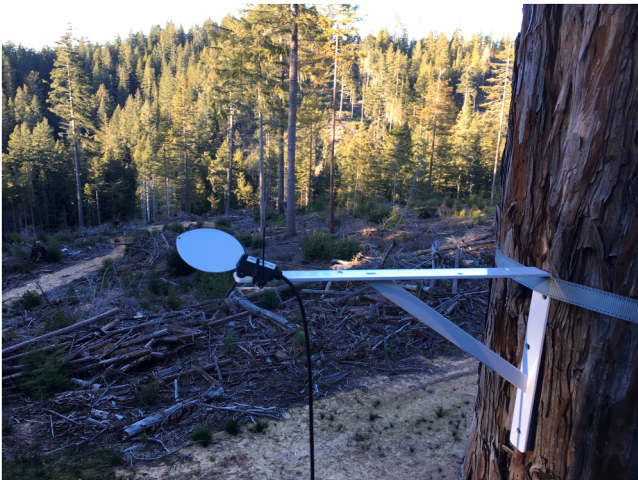
Fig. 2. Photograph of leaf wetness sensor (LWS) secured to a bracket and mounted at a height of 6.1 m in a S. sempervirens tree at the harvested ridge site.
