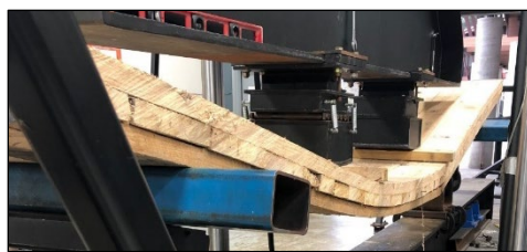
Figure 7.12 —Freshly manufactured green oak three-ply bolt-laminated mat during flexural testing. The span to depth ratio of the composite section is approximately 28:1.
