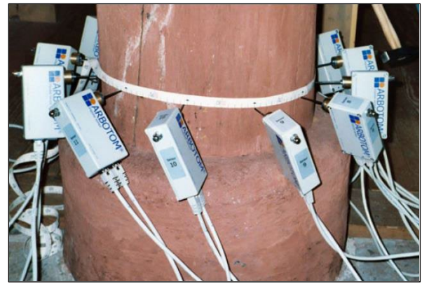
Figure 4.1—Acoustic tomography test on a timber post.
