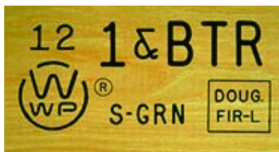
Figure 6.3—Grade stamp from WWP No. 1 & Better dimension lumber. Moisture content is surfaced green (unseasoned) condition, over 19% (WWPA 2021).
