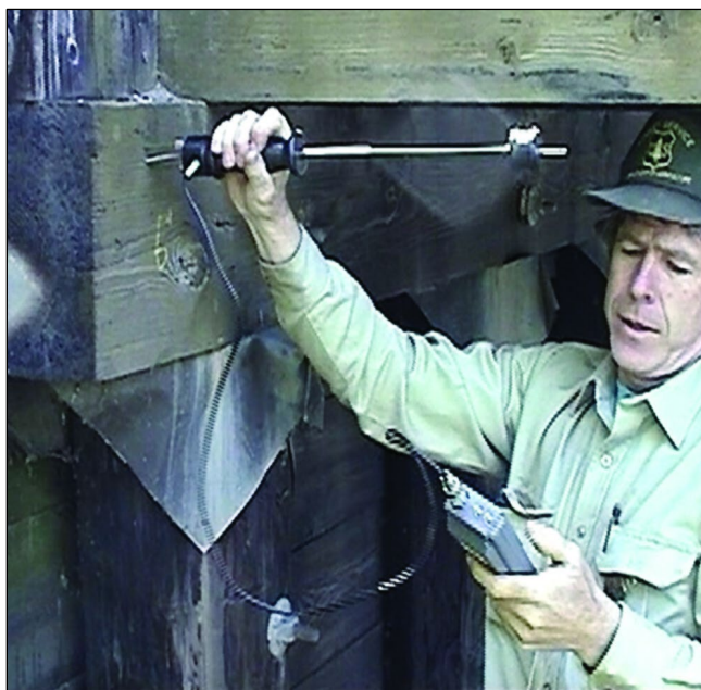
Figure 2.7—A pin-style moisture meter is used to determine moisture content of timber elements.
