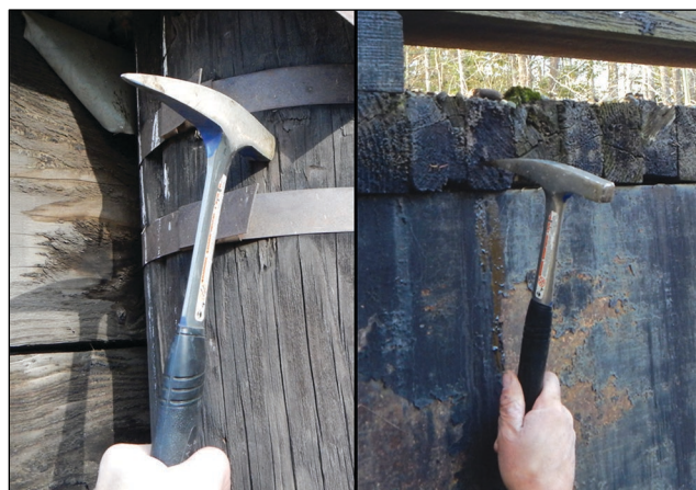
Figure 2.1—A hammer pick is an effective tool for initial assessments of timber bridge elements.
