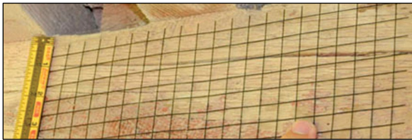
Figure 6.9—Use of grid to easily estimate the slope of grain. The 2:18 grids above implies 1 in 9 slope of grain. The black line shows the direction of slope of grain.
