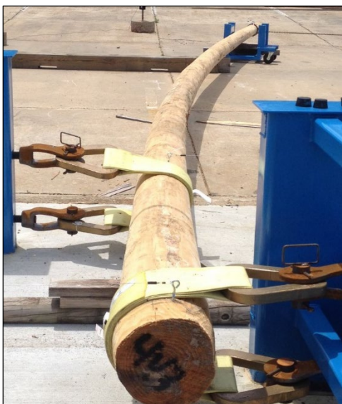
Figure 7.11 —A class 4, 40-ft Southern Pine utility pole during ASTM D1036-12 (ASTM 2018) flexural test. Per ANSI O5.1, Annex B (AWPA 2017), the minimum required tip load is 2,400 pounds, applied 2-ft from the end.
