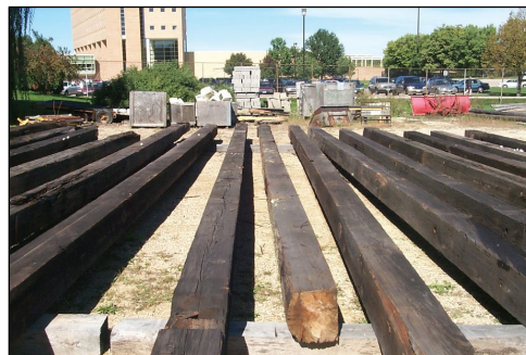
Figure 8.1—Fifteen 12- by 12-in. white pine timbers removed from the Quincy Mine Blacksmith Shop.
