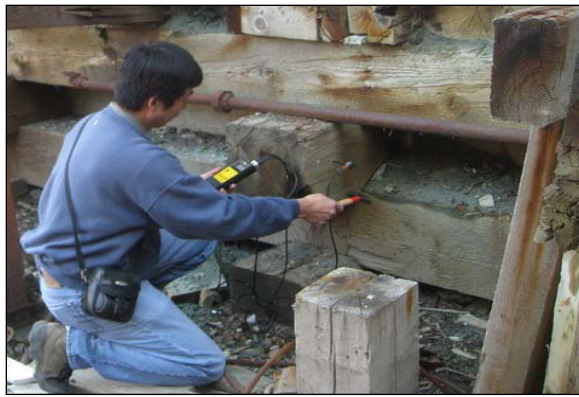
Stress wave measurements being conducted using a microsecond timer device.
