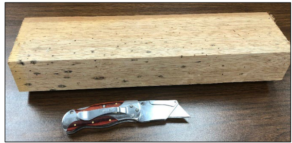
Figure 1.10—Beetle damaged section of a board. Note many of the holes show fungal staining about their perimeter. Also note, many of the holes / tunnels are not perpendicular to the surface of the board which indicates the holes were present in the log at the time the board was milled therefrom.
