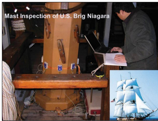
Figure 4.5—Inspection of the masts of the U.S. Brig Niagara using acoustic tomography.
