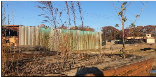
Figure 1.12—Flora, including a hardwood sapling, growing from the surface of a stack of wet timber mats. These mats are evidently decayed and ready to be stripped of their metal hardware, chipped, and used for mulch or boiler fuel.
