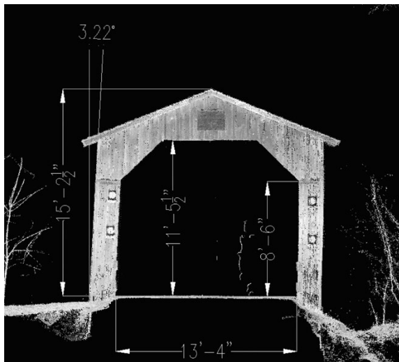
Figure 4.11—Dimensioned point cloud image of bridge entry on Cedarburg Bridge (SightLine, LLC).
