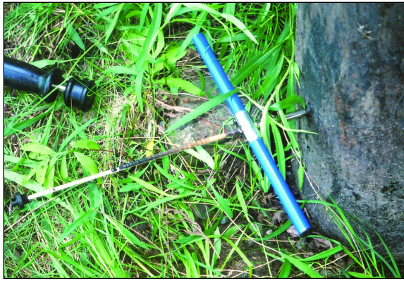
Figure 2.8—An increment core can be used to conduct inspections of timber bridge elements. This image shows an extracted core from an in-service timber pile ready for examination.
