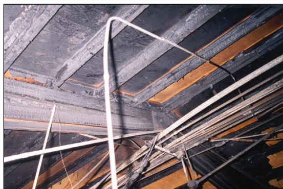
Figure 5.4—Charred and uncharred wood members in the Building 2 fire at the Forest Products Laboratory.
