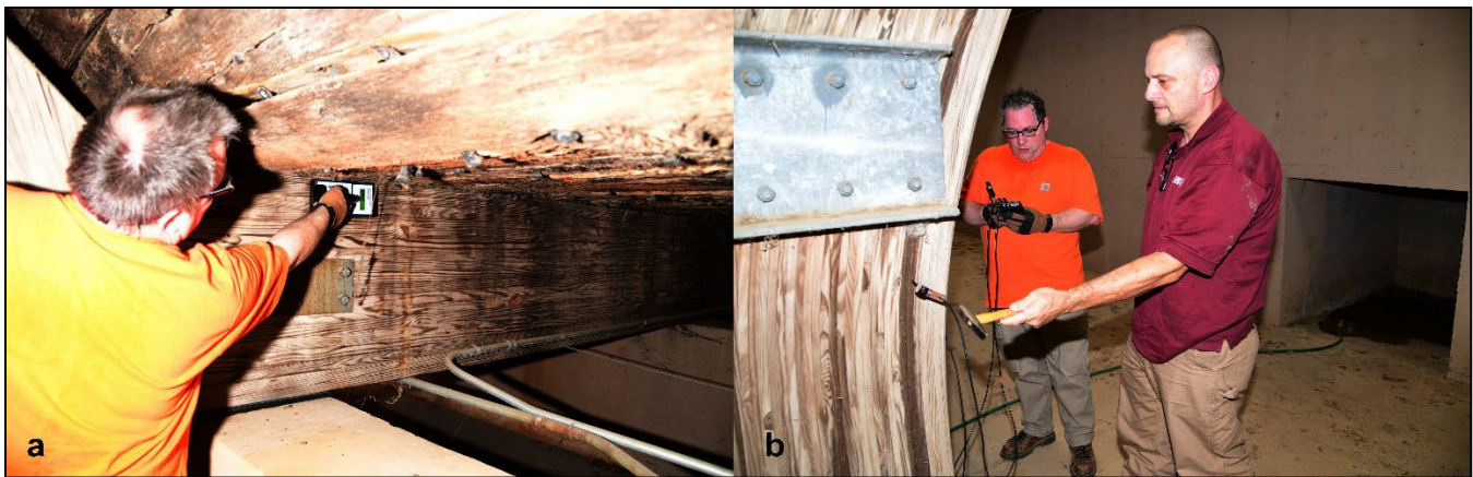
Figure 10—Inspection tools used on USS Cairo glulam structure: (a) Wagner L610 digital lumber moisture meter; (b) Fakopp microsecond timer.
