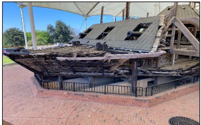
Figure 1—USS Cairo in Vicksburg National Military Park on display outdoors under a canopy and supported by a glulam crib structure.
