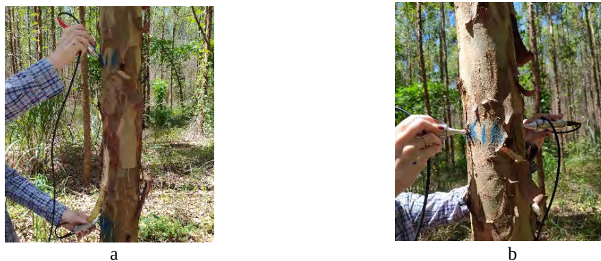
Figure 2. Ultrasound tests being carried out on trees with indirect measurements (transducers positioned on the same face) (a) and direct measurements (transducers on opposite faces) in the radial direction (b).
