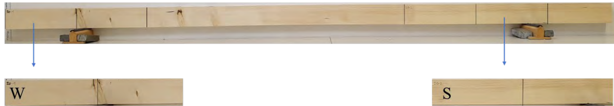
Figure 3 — Visual identification of the weakest (W) and strongest (S) cross-section in a sawn timber board from which the characteristic weak (W) and strong (S) small test specimens ( L = 700 mm) were cut out.
