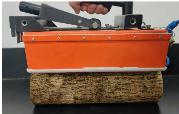
Figure 1 —Illustration diagram for detecting moisture contents of wood discs using tree radar.
