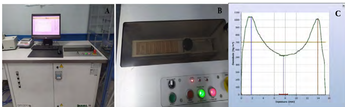
Figure 1 — X-ray densitometer (A); specimens at the time of testing (B); graphic result of the panel density profile (C).
