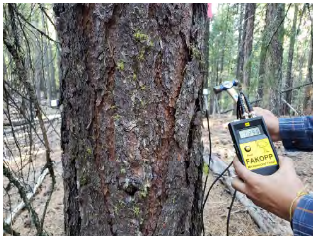
Figure 1. Transverse acoustic measurement conducted at the breast height of a tree sample in two perpendicular directions: north-south and west-east.
