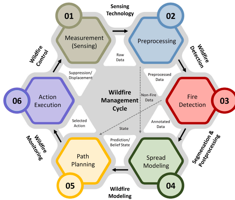
Fig. 14. The data flow cycle between modules involved in wildfire management: sensing, preprocessing and detection, modeling and planning, and control.
