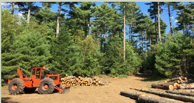
A cable skidder in an eastern white pine harvesting operation. Courtesy photo by Maren Granstrom.
