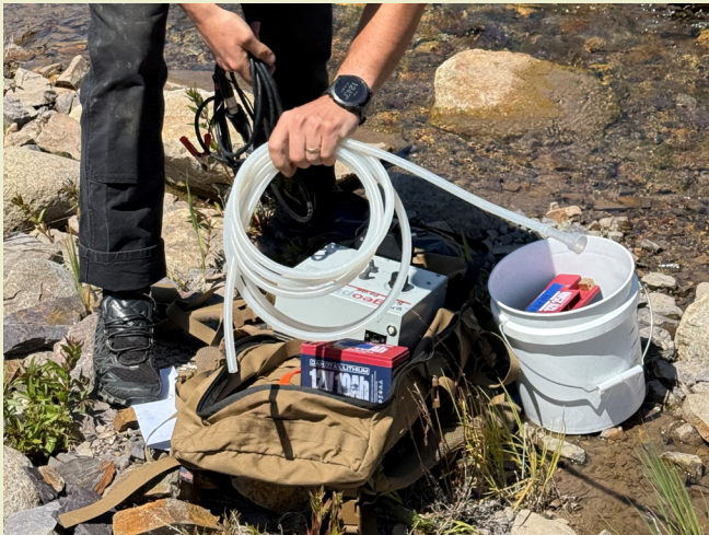
A scientist sets up an eDNA collection kit (a pump, tubing, a filter, and a bucket) on a stream bank. USDA Forest Service photo by Michael Schwartz.
