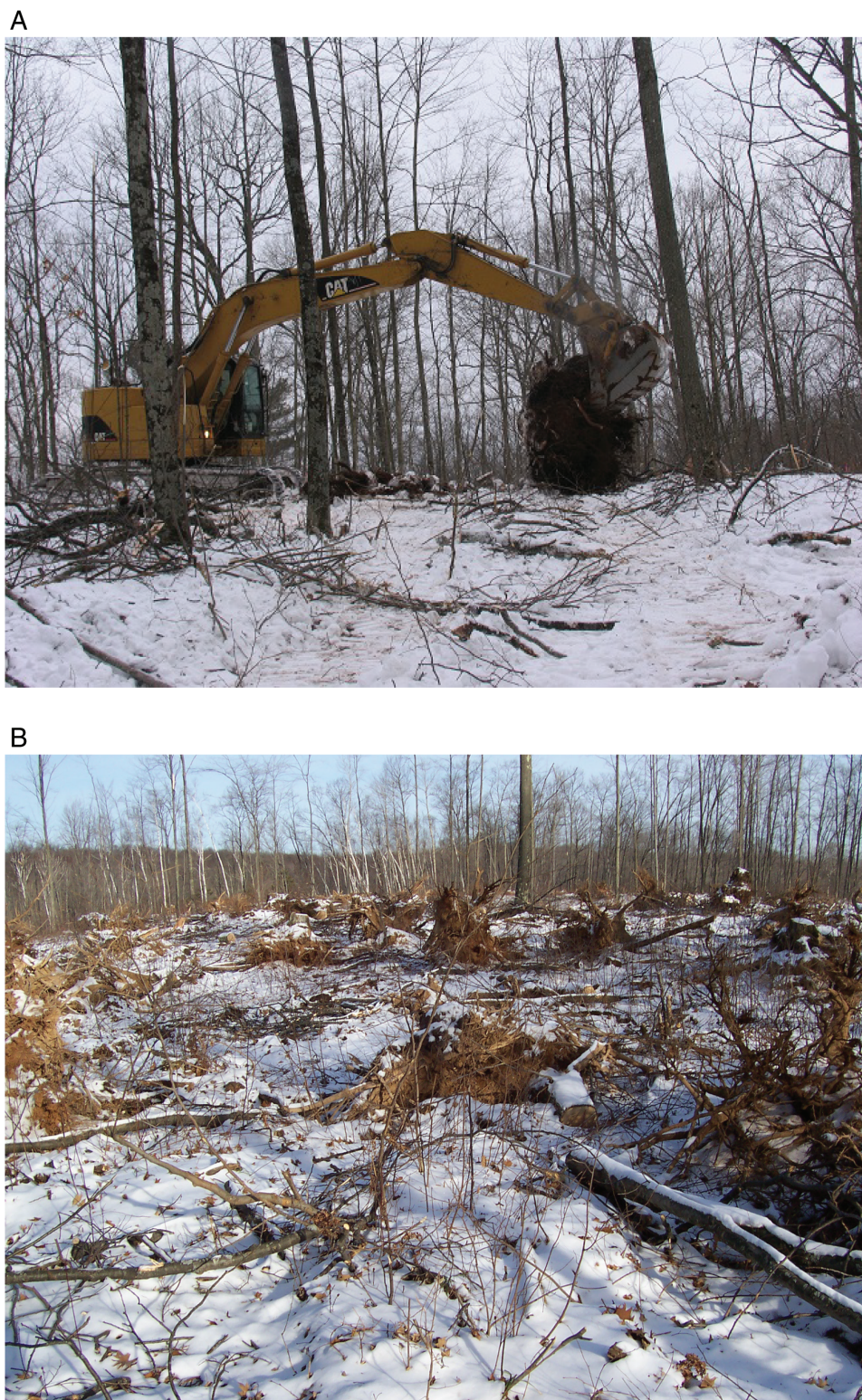
Figure 2 Root rupture treatments were implemented on the Chequamegon–Nicolet National Forest (CNNF) and Menominee Forest (MF) during winter months before March 15. Q. rubra trees (>4 in. DBH for CNNF; > 5 in. DBH for MF) were harvested and the stumps and root masses were dug out with an excavator. The excavator was equipped with a narrow bucket (frost bucket) that is used for digging into frost and/or compacted soil and thumbs for grabbing stumps. A) Photo from the MF of stump and root mass being pulled from the ground and flipped upside down. B) Photo from the CNNF of an oak wilt infection center after completed root rupture treatment.
