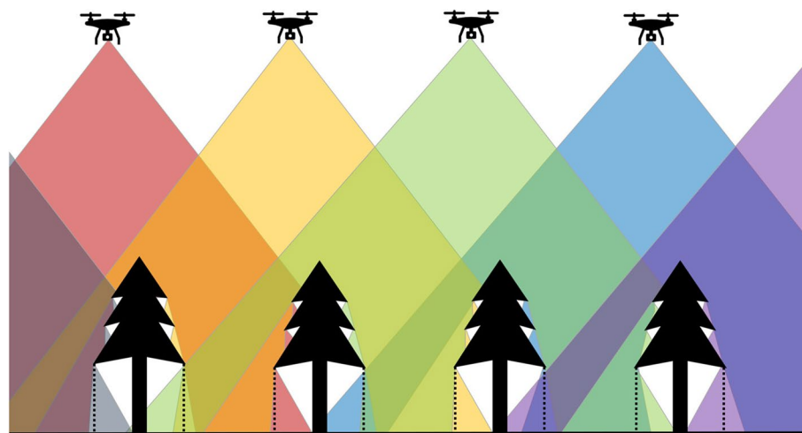
Fig. 1 Conceptual diagram of the area occluded from nadir imagery (denoted by the dashed black line). In this diagram, approximately 50% of the ground is occluded by the trees, but the entire ground is captured from the oblique views from the drones. The field of view from the drones is \sim 80^\circ with \sim 80\% overlap. These are common values for drone image acquisition
