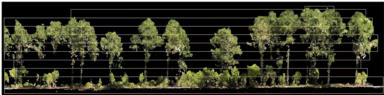
Fig. 4 Two-meter height strata highlighted in one of the height normalized RGB photogrammetric point clouds
