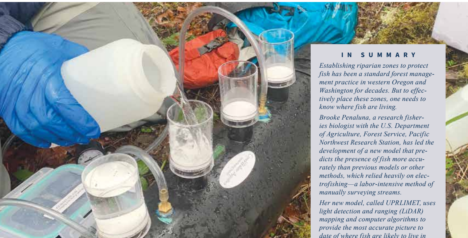
A researcher pours stream water into an environmental DNA filtering system. With this system, researchers can simultaneously process four samples from one site. The replicate samples increase the ability to detect target species at a site. USDA Forest Service photo by Laura Hauck.
