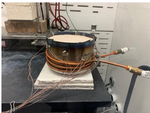
Fig. 5. Cooling the samples. Pyrocosm with sand-PyOM matrix is wrapped in water-circulating ring. Thermocouple wires can be seen attached to the pyrocosm.
