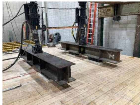
Figure 5 Load Placement used for Transverse Panel Deck Tests
