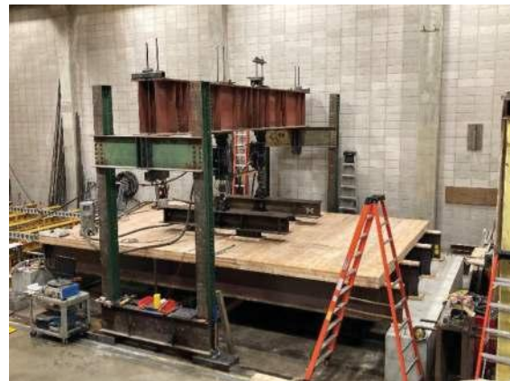
Figure 4 Example of Transverse Panel Test Configuration
