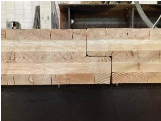
Figure 1 Panel Edges Joined with Half-Lap Joint
