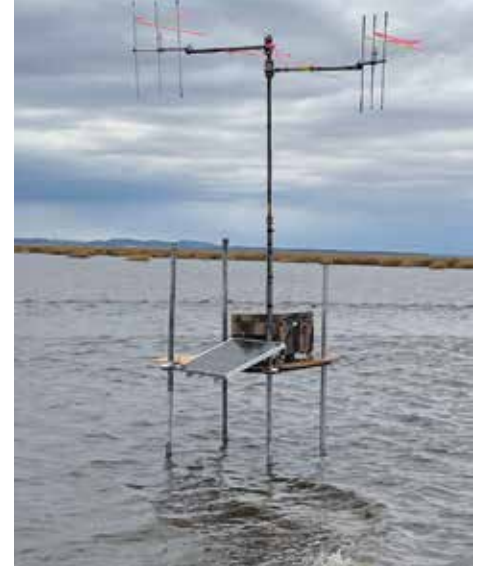
A monitoring station in Malheur Lake used for monitoring water quality and tracking carp via radio telemetry. Photo by James Pearson.
