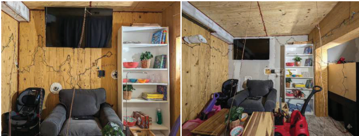
Figure 2: Varying amounts of exposed mass timber in back portion of Test #2 (left) and Test #3 (right) prior to testing.
