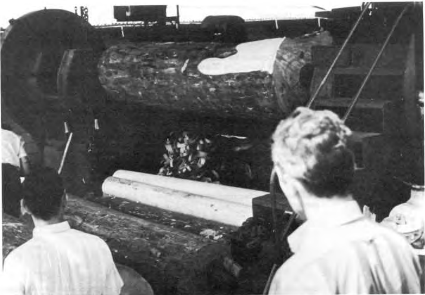
Plywood mill in San José, Costa Rica, produces rotary-cut veneers mostly from banak ( Virola spp.) and crabwood or cedro macho ( Carapa guianensis ). Logs trucked in from the Caribbean coast.
