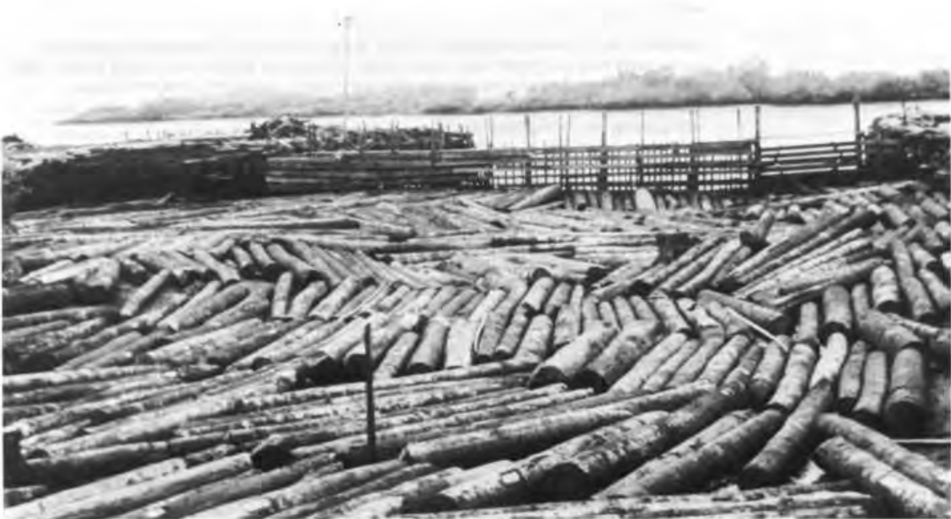
Highly perishable cuangare ( Dialyanthera spp.) and banak ( Virola spp.) logs harvested from coastal lowlands in southwest Colombia are ready for pond storage
