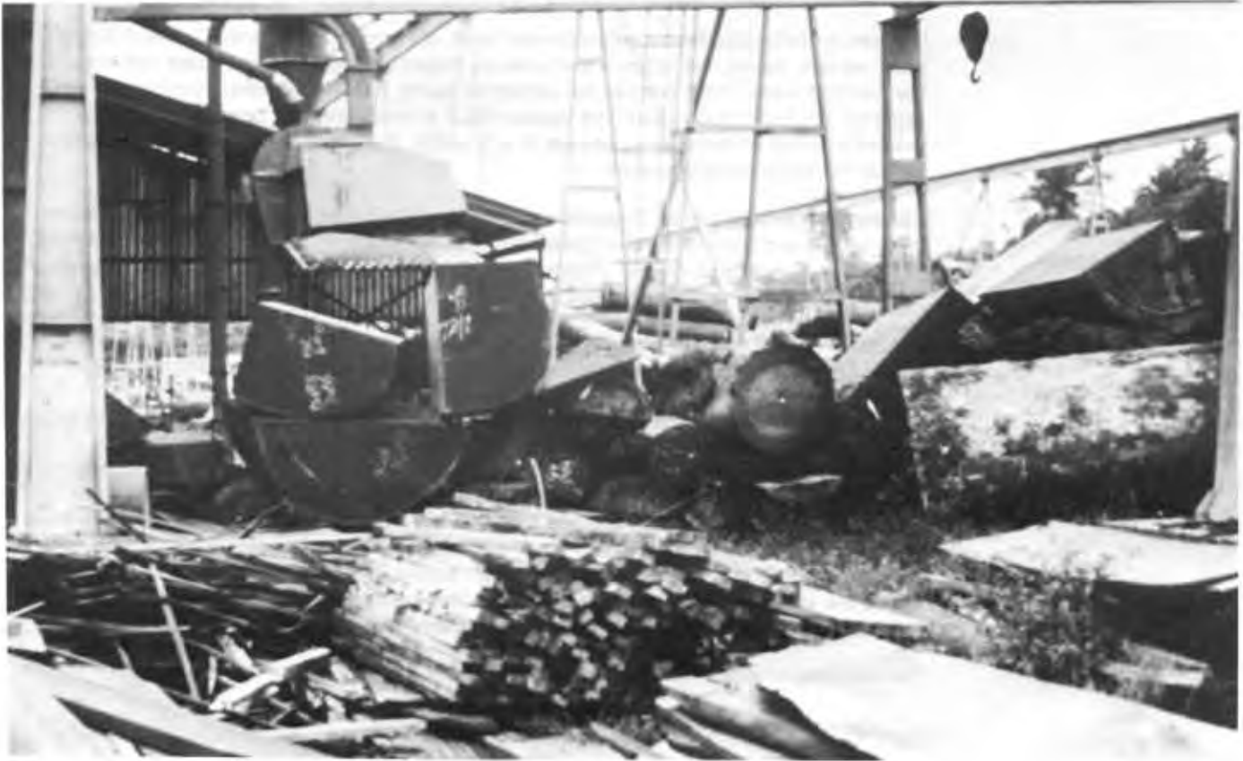
Unless processing complexes are integrated, much of the log, as at this Nigerian mill, ends up as residue—a universal problem.
