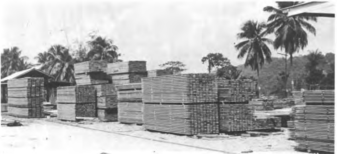
Degradation of wood products due to attack by decay fungi and insects is an ever-present hazard in the tropics. Construction lumber imported into Puerto Rico is treated with wood-preserving salts and then stacked for air-drying.
