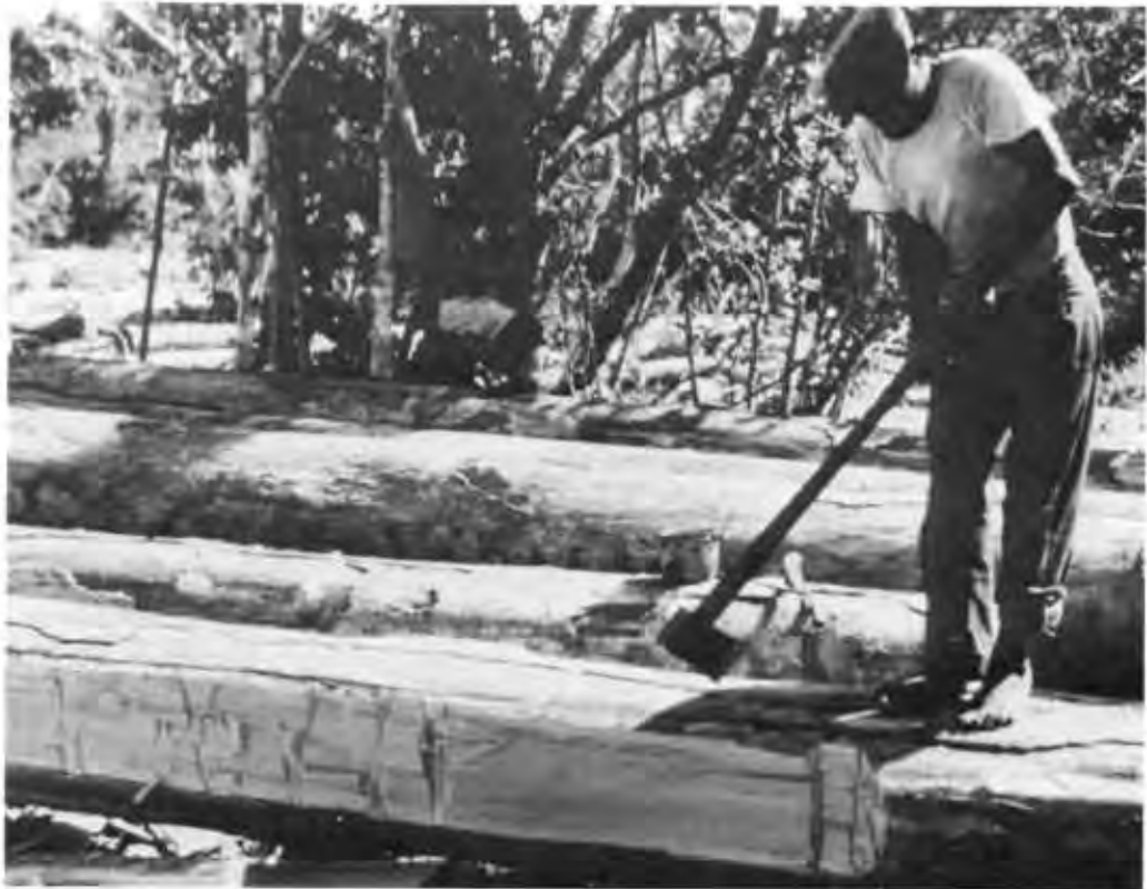
Some European markets still prefer hand hewn greenheart ( Ocotea rodiaei ) for heavy marine construction. Work is being done on a river landing in Guyana.
