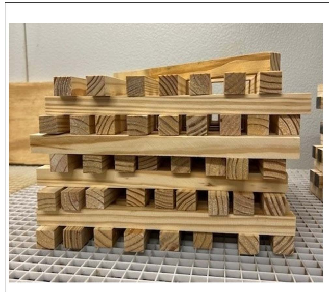
Figure 1.—Toughness specimens from time 0 after machining and before toughness testing.
