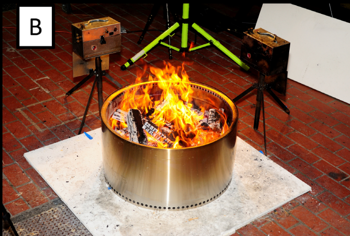
Figure 5 —Diagram and photos of the experiment setup on the combustion chamber floor. (A) Aerial schematic of locations for fire pit, background CO 2 measurement and radiant heat measurements. (B) The Solo fire pit during testing. (C) The Solo fire pit and combustion chamber exhaust stack during testing. USDA Forest Service photos.
