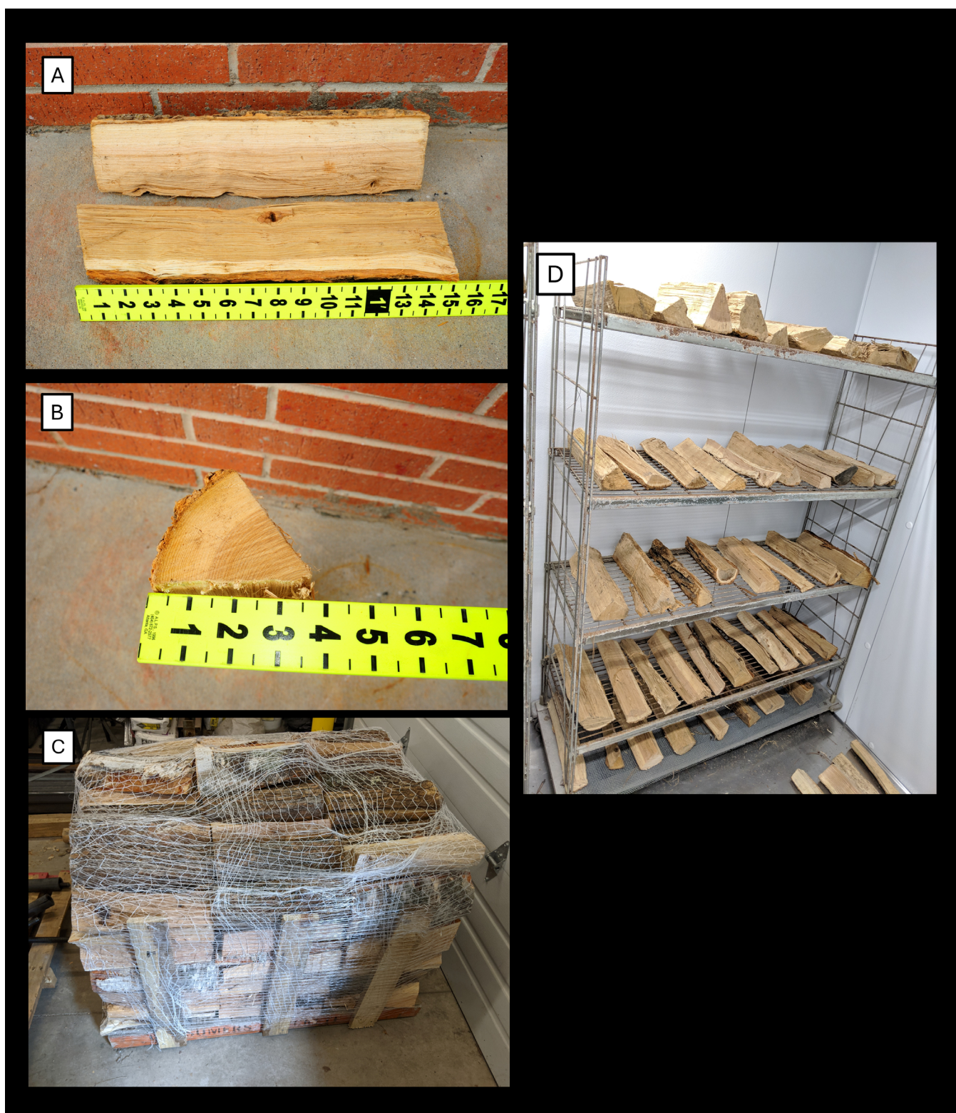
Figure 3 —Firewood used in testing. (A) Split firewood log, (B) split log, (C) face cord of split firewood, and (D) firewood being conditioned in the FSL environmental chamber.
