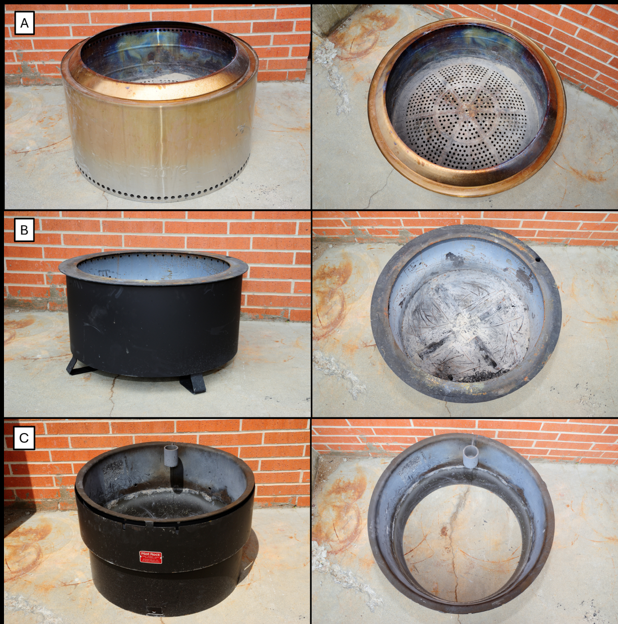
Figure 2 —Fire pits post testing. (A) Solo, (B) Breeo, and (C) Pilot. Fire pit heights (H), diameters (D), and volumes (V) are Solo: H = 43 cm (17 inch), D = 69 cm (27 inch), V = 0.16 m 3 (5.6 ft 3 ); Breeo: H = 41 cm (16 inch), D = 61 cm (24 inch), V = 0.12 m 3 (4.2 ft 3 ); Pilot: H = 46 cm (18 inch), D = 81 cm (32 inch), V = 0.13 m 3 (4.6 ft 3 ) after accounting for 20 cm of sand (see section 2.2).
