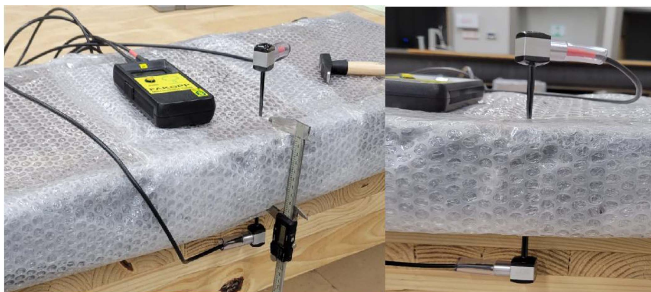
Figure 3.—Exemplar of measuring the distance and flying time on the lignin-foam block.
