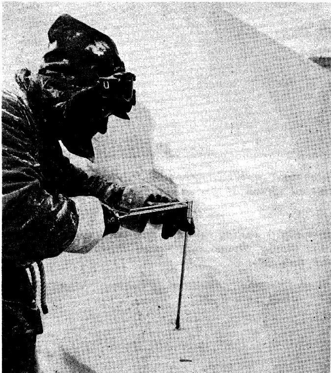
(Upper left) M. Martinelli, Jr., testing snow strength with a torque wrench and vane; (below) Elnora Martinelli, obtaining snow sample to determine water equivalent.
