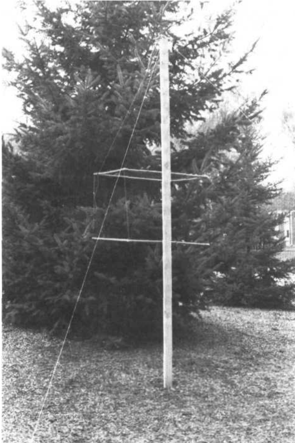
Figure 1. — Single-branch enclosure installed 2 meters above ground.
