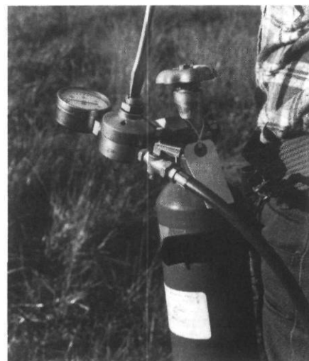
Figure 3.—Small-plot CO 2 research sprayer: A Complete apparatus ready for use; B Bottle with spray head attached and carrying case on left; C Stainless steel 50-mesh strainer and check valve assembly; D CO 2 cylinders in transporting box (cylinders must be kept upright); E Adjustment of pressure regulator (see text).
